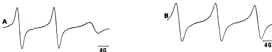
Fig. 4. A. Polyamide IIIa in m -cresol. B. Polyester IVa in chloroform ( T = 297^\circ\text{K} ).
